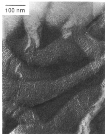
Figure 7. Electron micrograph from a replica taken from a freeze-fracture surface of melt-crystallized F(CF_2)_{12}(CH_2)_{14}H ; width of the stripes is 5 nm.
